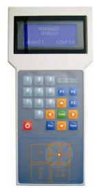
Numerical keys 1,2...0: F1 F2 F3 function keys: Arrow keys: Enter key: Esc key: Canc key: Red key: characters insertion programming operations cursor shift data confirmation exit from the menu inserted data deletion turn on/off
