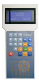
Numerical keys 1,2...0: characters insertion F1 F2 F3 function keys: programming operations
