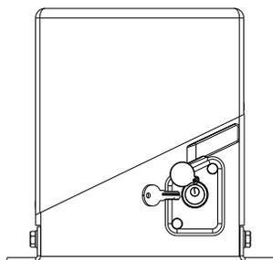
Rotate the unlocking device cover and put the key into the cylinder
