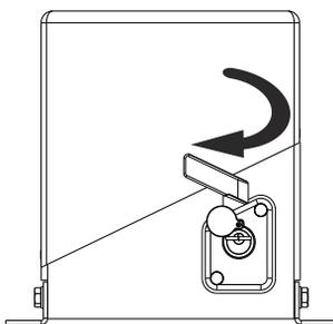
Rotate the unlocking device of 180°
