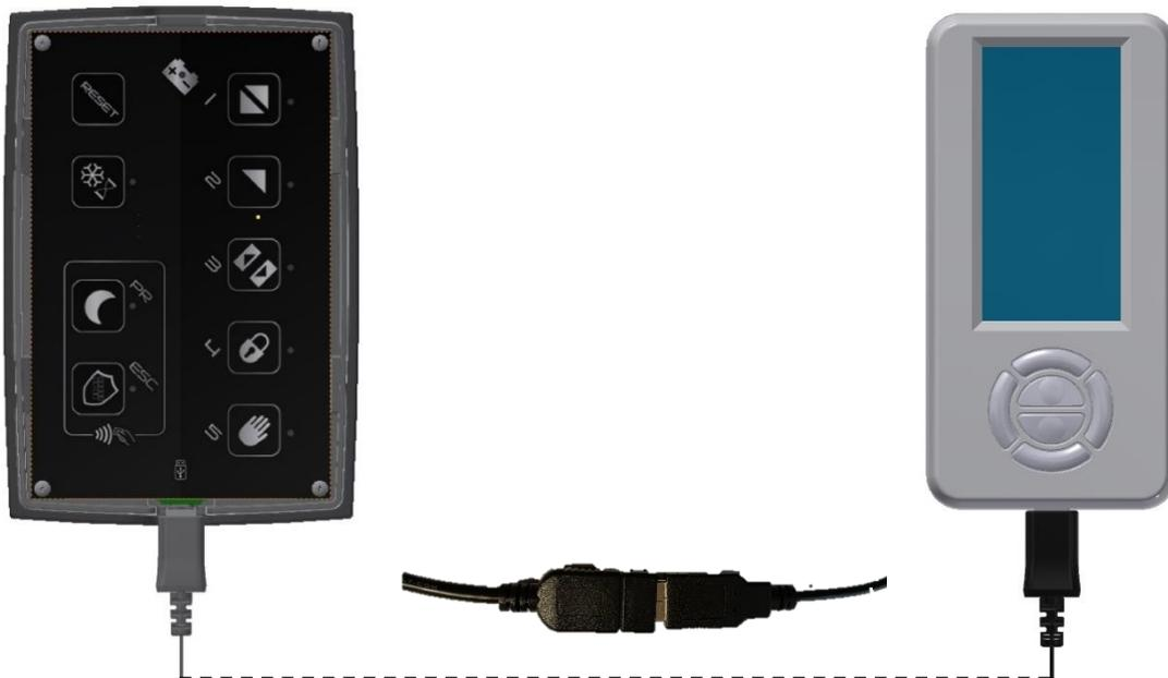
The micro-usb port is for exclusive use for the connection, using commercial cables not supplied, of the Digidor or Digidor T or Digidor BT (EXCLUDING BLUETHOOTH FUNCTION - NOT WORKING). Once connected, the Digidor will be functional and usable (for functionality see Digidor manual).
