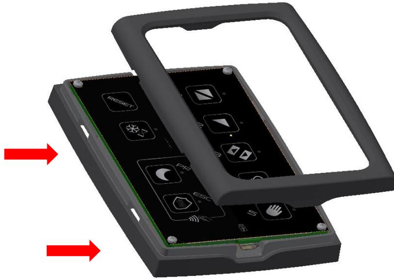
In order to access the micro-usb port, remove the front cover by using a screwdriver in the appropriate clicks indicated in the figure with arrows.
