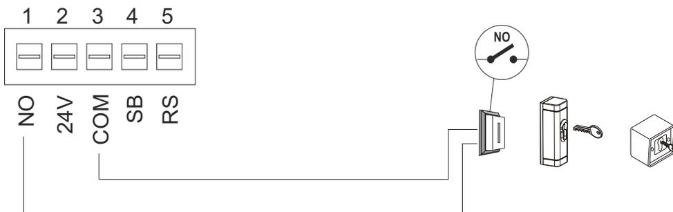
**14** Collegamento FOTOCELLULE / PHOTOCELLS connection
