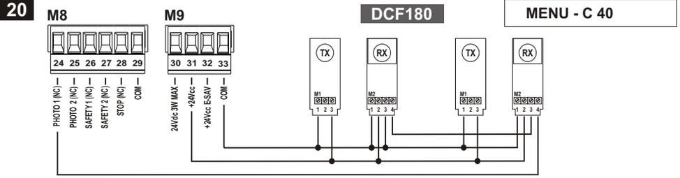
PHOTOCELLS 1 WITH TEST CONNECTION
