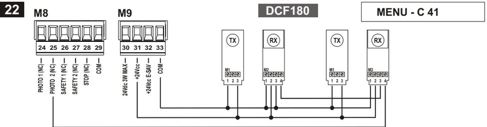
PHOTOCELLS 2 WITH TEST CONNECTION
