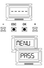
With control unit at rest press the buttons (ESC and OK) at the same time for 3 seconds, it will immediately appear MENU, then PASS.
