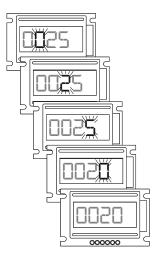
Press the button (OK), the second digit will start blinking. **WARNING** In this phase the button (ESC) is not enabled.
