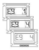
Press the button (OK), the display will start blinking **WARNING** In this phase the button (ESC) is not enabled.
