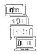
The second digit will blink, use the button ( + ) till display the number (2). Press the button ( OK ) to confirm
