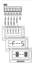
The contacts of terminal M8 are multifunction and can be programmed with menus C40-C41-C42-C43-C44, in the manual they will be identified with the name of their default or primary function.
