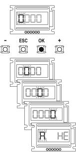
Make the access to the programming as described in chapter 11. Press the button (OK) to confirm.
