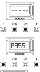
It is possible to make a reset of the control unit to come back to factory parameters.
