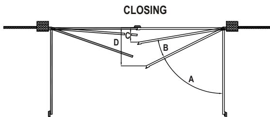
A = Normal movement with security devices intervention and motion inversion
