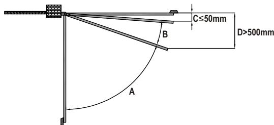
A = Normal movement with security devices intervention and motion inversion
