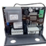
2B AS07300 Control unit with on-board radio receiver (SR302 - 868 MHz)
