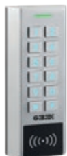
DCD300 Keypad with card reader, vandal-proof, surface-mounted, IP66, 2 relays, 999 codes / keys, 12-28 Vac-dc with 2m cable
