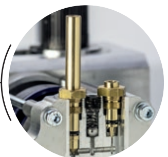
SPEED ADJUSTMENT VALVES AND MANUAL RELEASE
