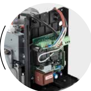
SC130 CONTROL UNIT WITH EMBEDDED RADIO RECEIVER
