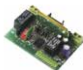
5 AU02910 2 channels plug-in receiver board for control units
