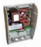
2 AS07000 Control unit with embedded radio receiver (SR2)
