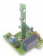
DSL230L 230 Vac LED spare flashing lamp card Code AU02610
